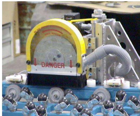
Photo of Deletion Wheel and Dust Collection Enclosure on a Table Deleter. Photo courtesy of ALKAB Contract Manufacturing.
